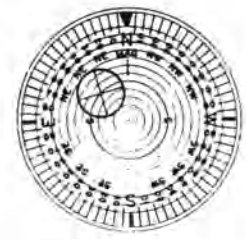
Fig. 8.43—Pendulum suspended inclinometer and compass unit for a 0 to 17° single-shot unit (after Eikelberg et al. 3 ).
