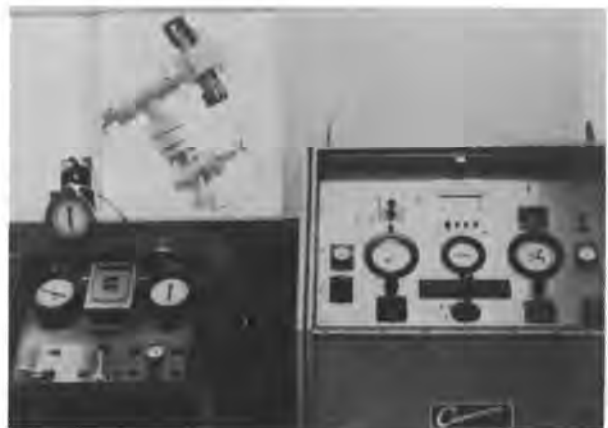
Fig. 1.53—Example control panels for remote adjustable choke.
