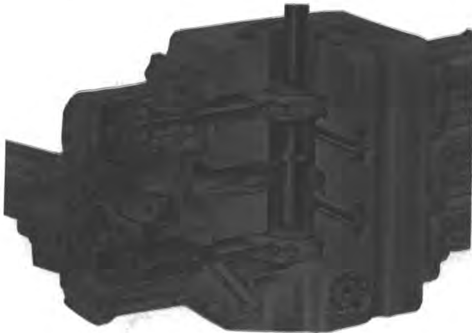
Fig. 1.43 – Example ram-type blowout preventer.
