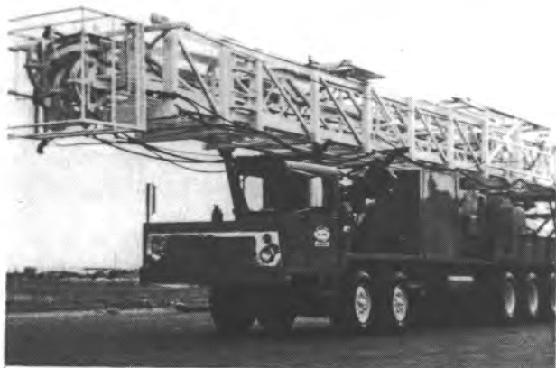
Fig. 1.7—Portable mast being transported.
